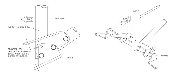
3. **MODIFY TAIL SPRING MOUNT PLATE:** Remove Mount Plate from Tail Spring. Modify Tail Spring Mount Plate per **FIGURE 130-3**. A new Tail Spring Mount Plate (KPTG0032) may also be purchased from RANS Parts Department.
