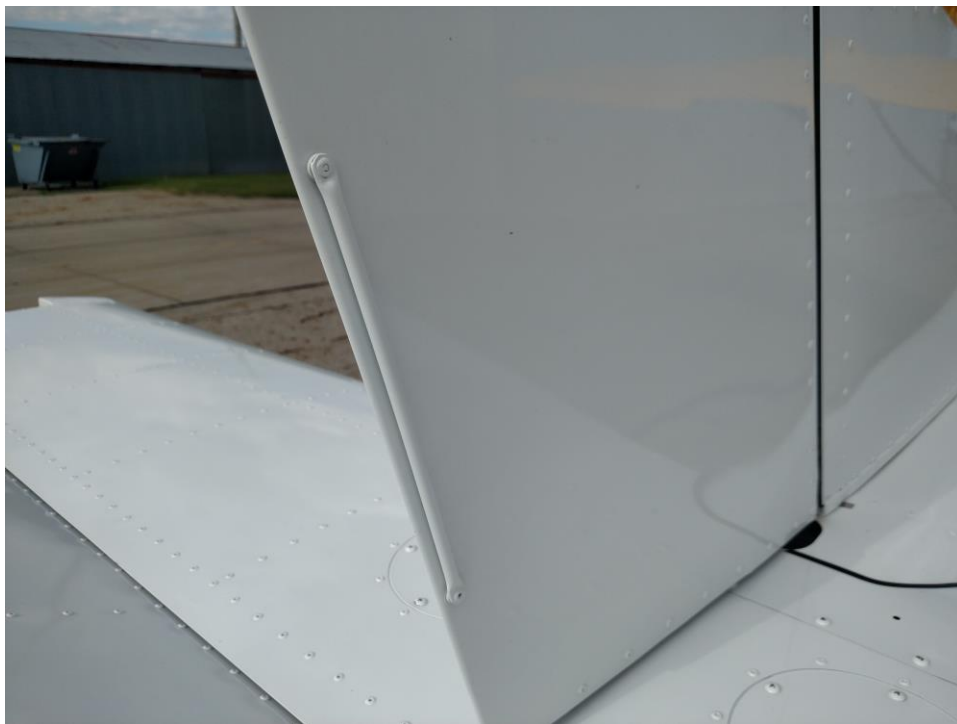
Permanent bump trim using 1/4" Aluminum tubing.
