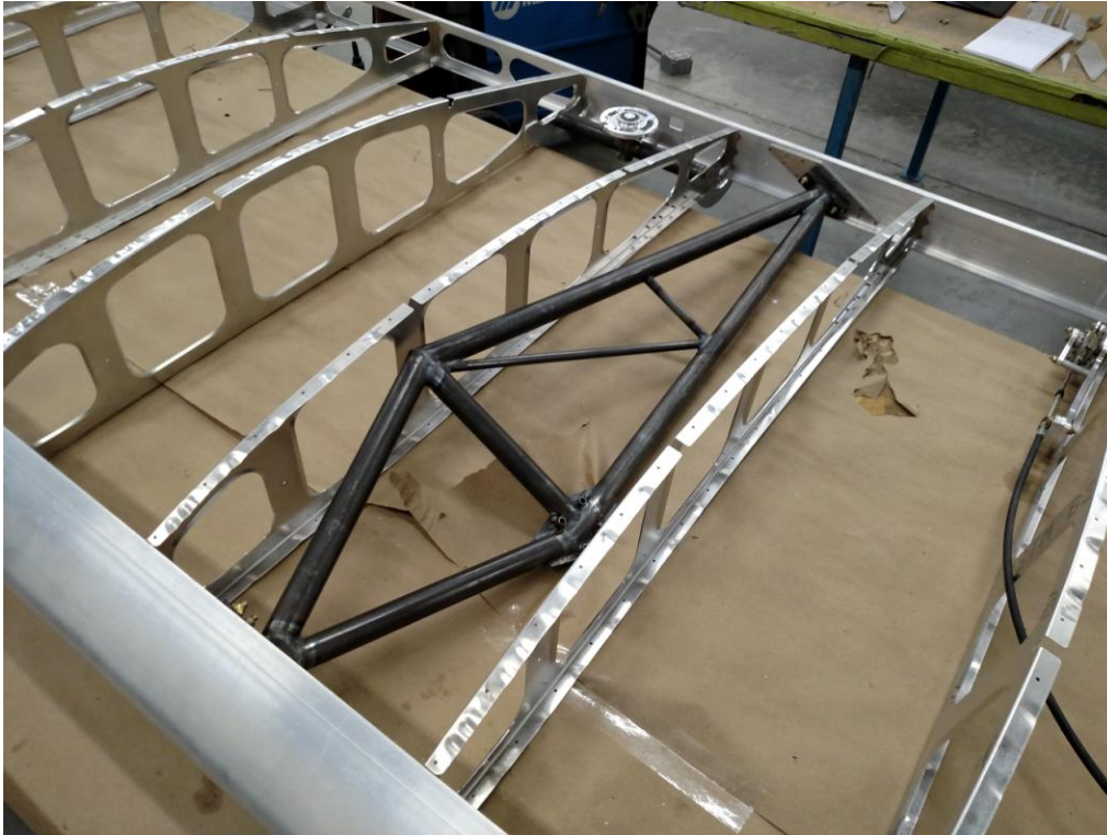
Wing truss bolts into the wing at the exact strut load path angle.
