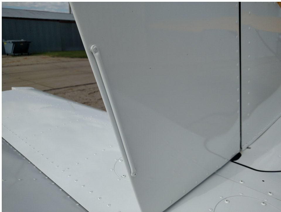
Permanent bump trim using 1/4" Aluminum tubing.
