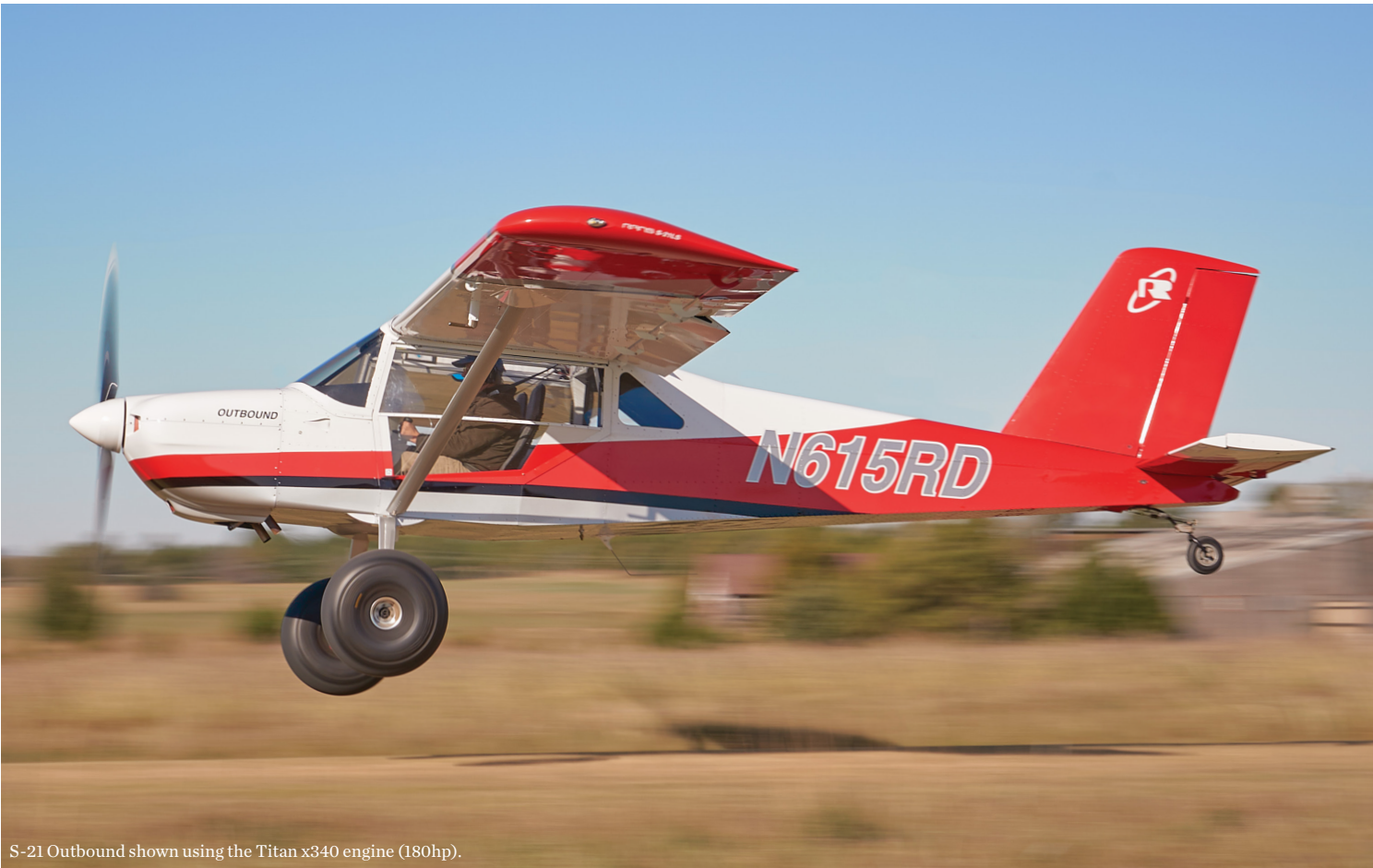
S-21 Outbound shown using the Titan x340 engine (180hp).
