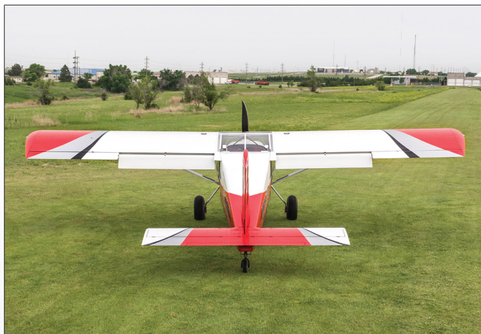
Large tail surfaces assure positive control at low speeds and great yaw and pitch stability. Electric pitch trim is standard.
