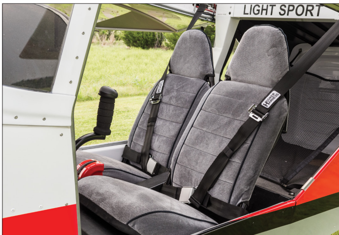
Seats are high on comfort and low on weight. They also adjust fore & aft in flight and have 4 recline settings. Optional headrest shown.
